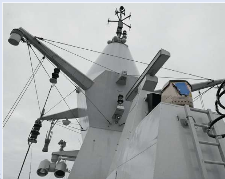
Système de veille infrarouge VAMPIR NG. VAMPIR NG InfraRed Search and Track (IRST).
