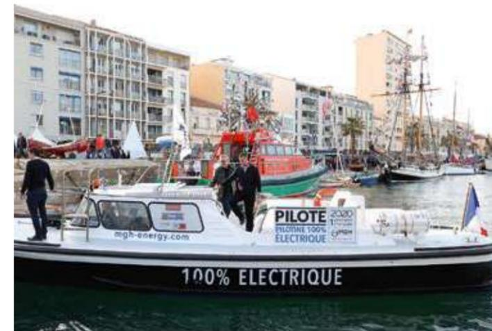
By initiating the Green Pilot project in 2018, the French company MGH has made it possible to develop the first 100% electric pilot boat from the conversion of the original diesel-powered Maguelonne pilot boat. Commissioned in spring 2021 at the Port of Sète, the E-Maguelonne pilot boat is now equipped with a 200-kW electric engine that
